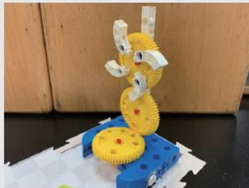
Diagram of a self-made windmill-device (can be modified by teams, but the windmill must be driven by the central output gear of the robot).
